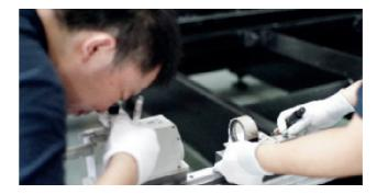
A collimator is run along the full length of the guide rail, testing for straightness. As required, micro-adjustments are made to ensure linear accuracy is achieved before shipment.
