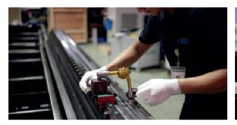
The use of an interferometer records the machines x and y axis movement during cutting to ensure accuracy.
