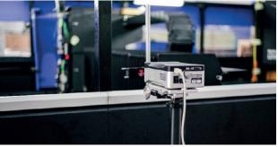
A Marble Test is performed to measure the x and y axis, calculating any necessary adjustments to ensure perfect level and alignment along the length of the machine.
